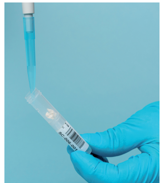
8. Add 100-150 \mu l elution buffer/cm serum paper, depending on the LOD of the analysis.
